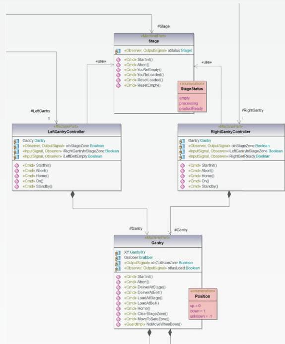
Detail of the static model that describes the relationships between the controllers of two linear robots ('gantry').
