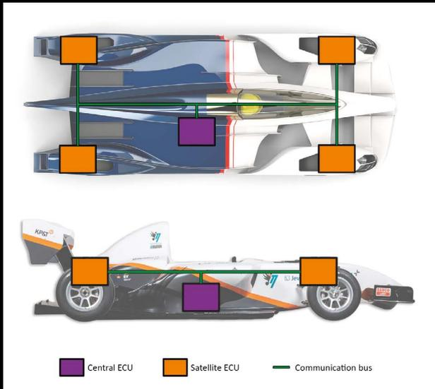
Figure 1: The IM01 will feature one central ECU and four satellite controllers, one at each corner of the vehicle.
