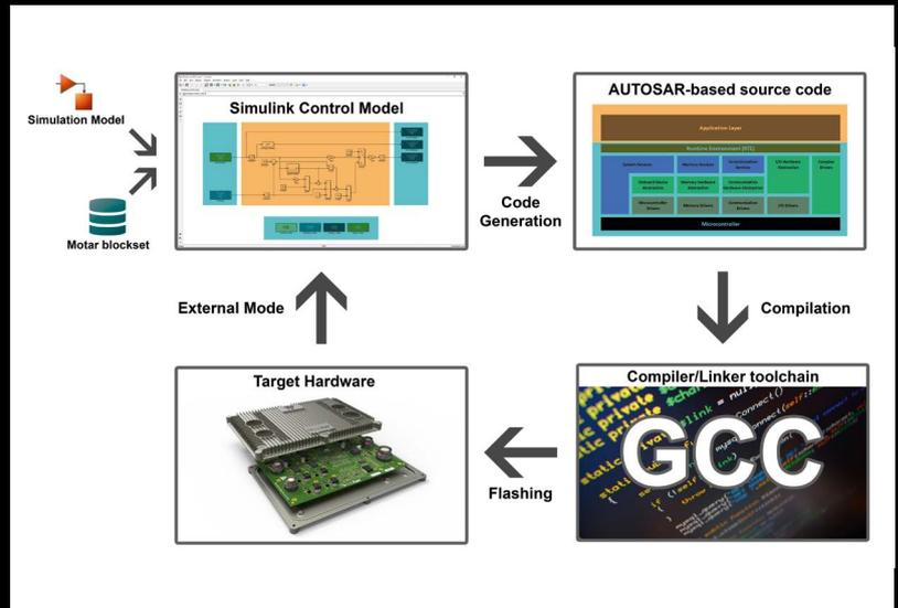
Figure 2: Using the Motar toolbox, the ECU software can be developed and deployed fully automatically.
